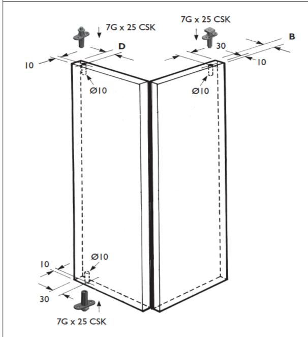
**i.** With a drill and 10mm drill bit, using the measurements above, drill 10mm holes into the appropriate positions in the door.
