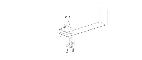
STEP 5: Attach guide to bottom of the doors (HF40 kits only)
