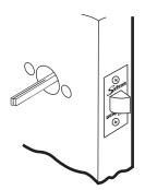
4 Drill and fit 4 wood screws for alignment only
