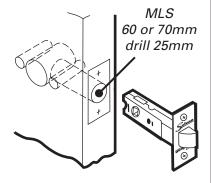
3 Fit spindle through latch
