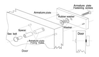
ARMATURE PLATES MUST BE FIXED AS SHOWN ABOVE.
