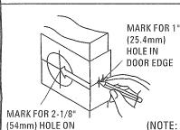
Start approximately 36" (914mm) from floor. Fold and apply template to edge of door and mark centre of door edge as indicated on template. Mark centre hole on door face through guide on template.
