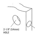
Drill 2-1/8" (54mm) hole through door face as marked for lockset. It is recommended that holes be drilled from both sides to prevent splitting. Drill 1" (25.4 mm) hole in centre of door edge for latch.
