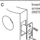
Insert latch and tighten screws.
